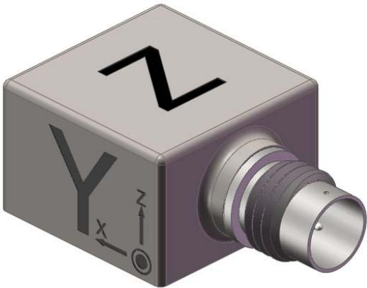
Model 3293A is a low-noise, high sensitivity, miniature LIVM triaxial accelerometer featuring a single, transverse mounted, 4-pin electrical connector. This feature allows the 3293A to be used in situations where vertical space is limited. Model 3293A is case grounded. The 3293A is a 500mV/g accelerometer.
